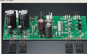
Dedicated power supply for signal input section
