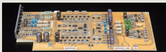
Balanced AAVA type volume control circuit
