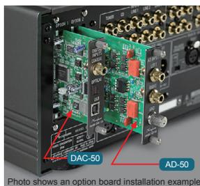
Photo shows an option board installation example.
