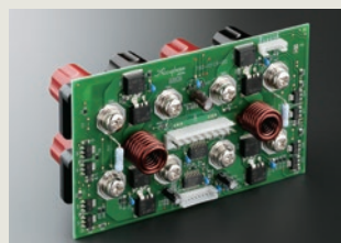
Protection circuitry with MOS-FET switches
