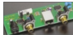
Assembly with transport outputs (HS-Link, coaxial) and digital inputs (optical, coaxial)
