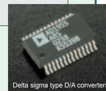
Delta sigma type D/A converters
