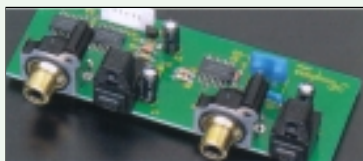
Assembly with transport outputs and digital inputs (optical, coaxial)
