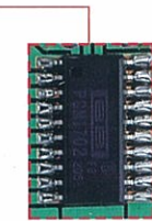
20-bit D/A converters (six units on rear side)
