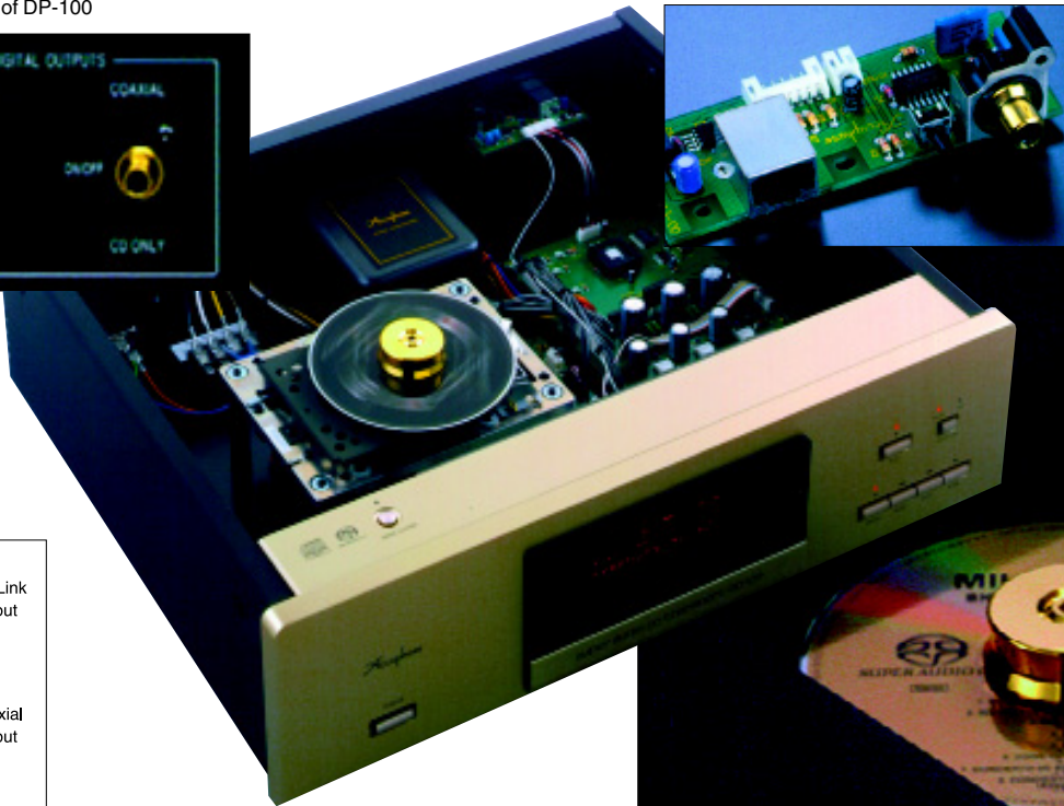
■ Assembly with HS-Link encoder, master clock generator, power supply circuitry, etc.
