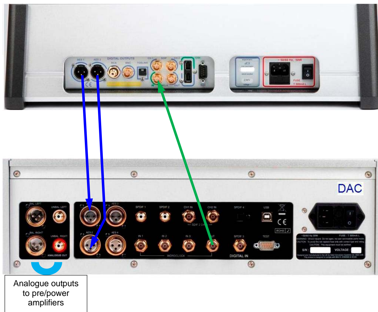
Figure 4 – Using the Scarlatti Transport with a Vivaldi DAC in Master Mode
