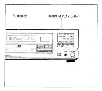
The DISPLAY button cannot be used during random playback. As tracks are randomly programmed by the CD player as random playback proceeds, the remaining playback time and elapsed playback time of the random program cannot be displayed.
