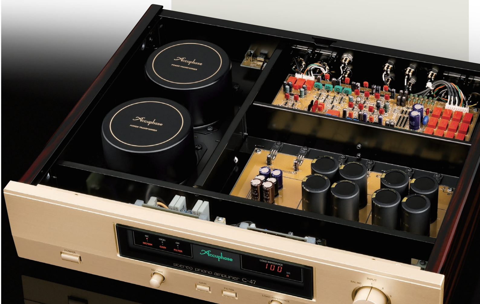
Internal layout realizes full mono construction to prevent mutual interference between channels
