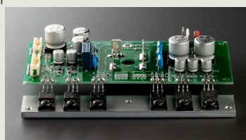
Dedicated power supply for signal input section
