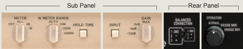
① Meter display selector ② Meter display range selector ③ Hold time selector ④ Input selector ⑤ Gain selector ⑥ Balanced input polarity selector ⑦ Operation mode selector
