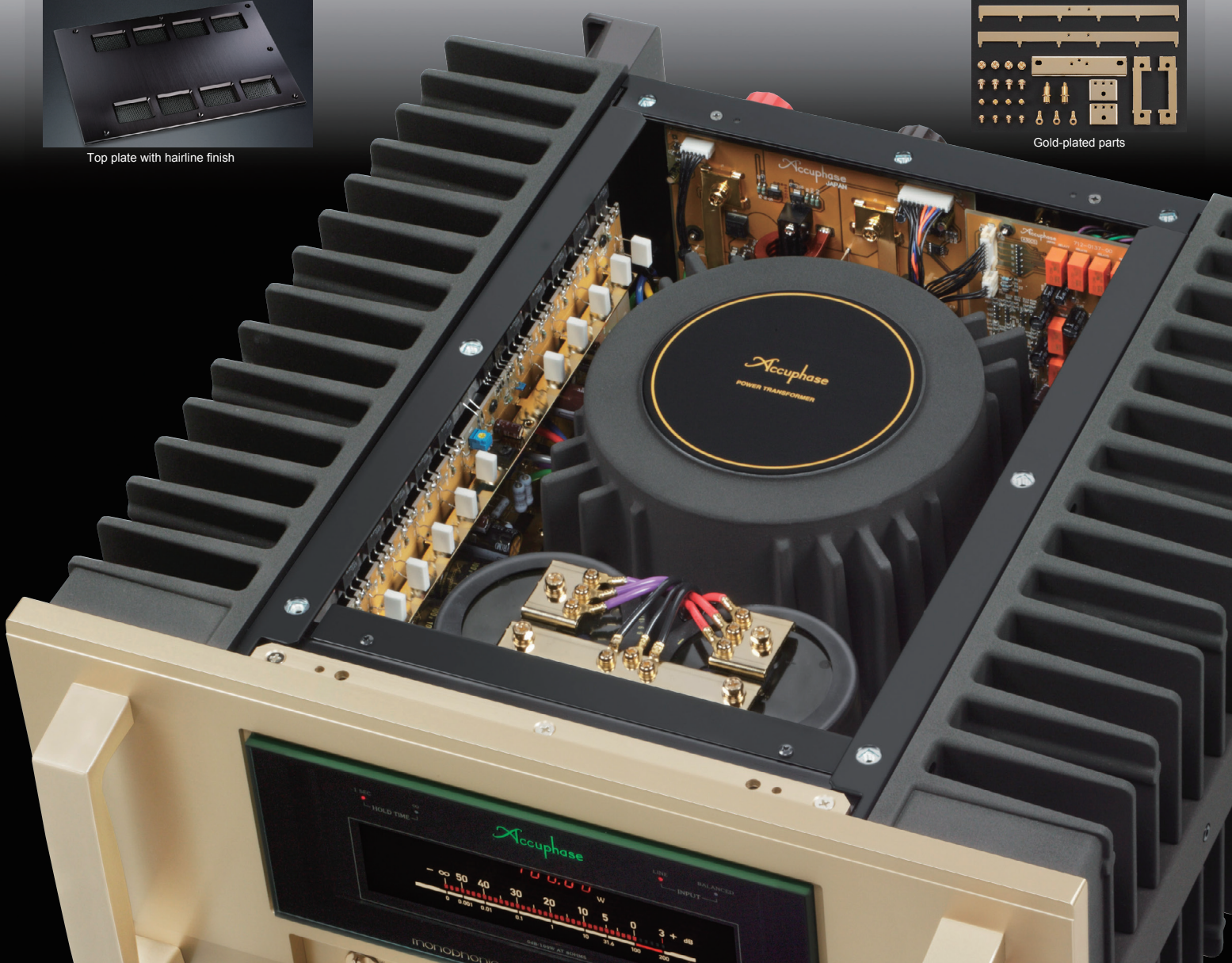
Large gold-plated speaker terminal made of solid brass
