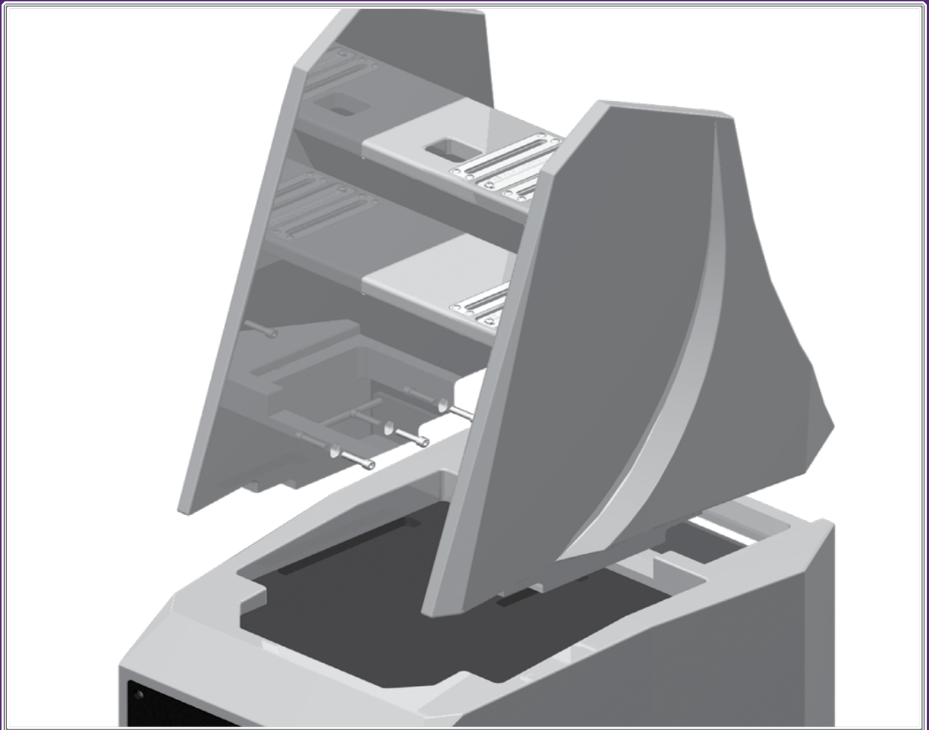
FIGURE 11 – CAREFULLY INSTALL WING ARRAY AND BOLT IT TO THE WOOFER MODULE.
