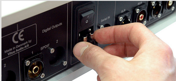
6. Position the new fuses vertically in the fuse carrier.
