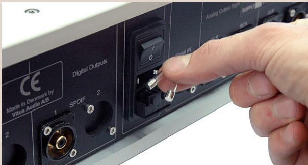
5. Fit new fuses into the fuse carrier.
