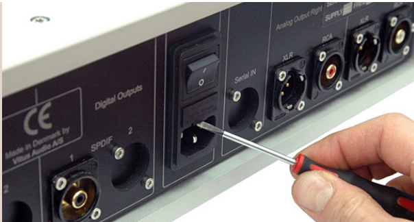
1. Take a small flat bladed screwdriver and place it under the fuse carrier.
