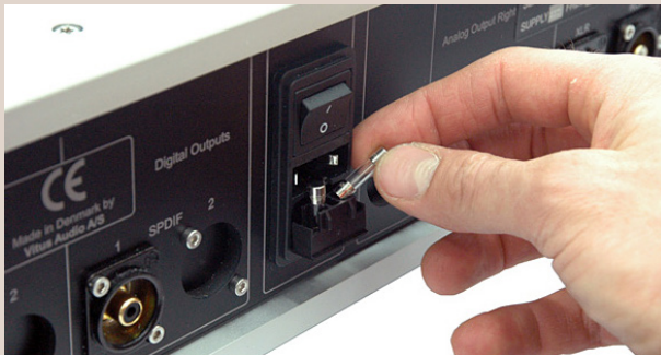
4. Remove the blown fuse(s).
