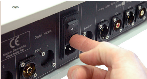
8. The fuse carrier is in place when you hear "CLICK".
