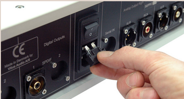
3. Pull out the fuse carrier.
