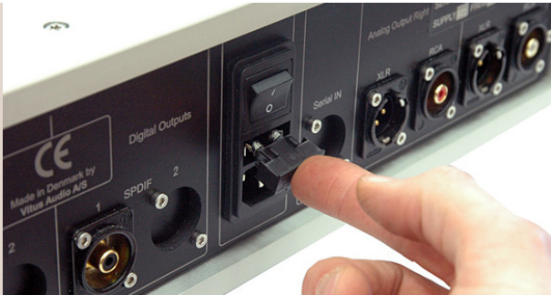
7. Push the fuse carrier back into the back of the MP-D201 Mk.III.
