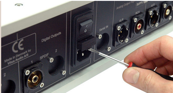
2. Open the fuse carrier.
