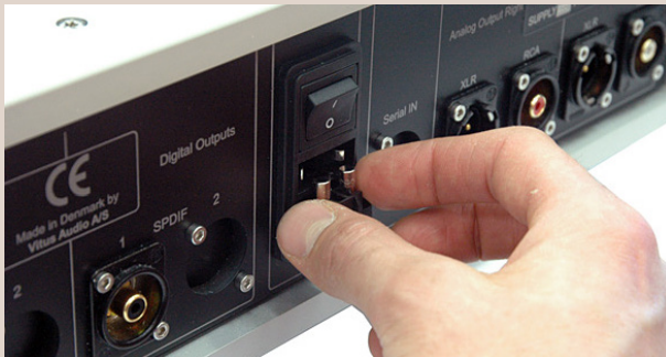
6. Positioned the new fuses straight-up in the fuse carrier.
