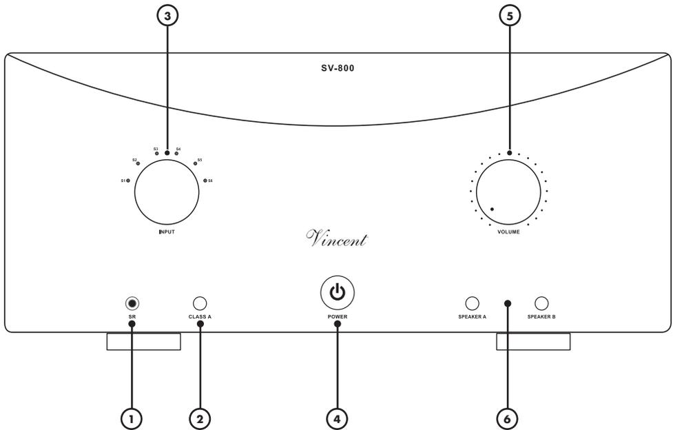
**1. SR: Infrared receiver for the remote control**
