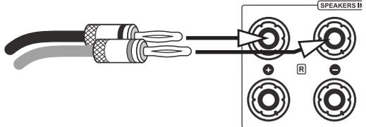
If no connector is to be used, remove approximately 1 cm length of insulation from each end of the speaker wire. Twist the braid in order to avoid short circuits. Turn the fastener on the loudspeaker terminal counter clockwise to loosen it and introduce the bare wire end into the exposed connector hole. Then turn the fastener clockwise so that the wire is firmly clamped. Make sure the connection is pretty tight.
