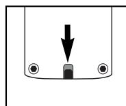
2. Remove the optionally used battery and correctly insert the new button cell, as schematically shown in the battery compartment.
