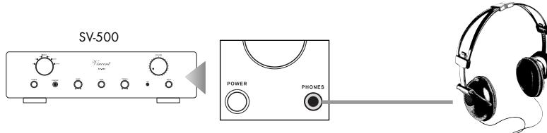
By doing this, the loudspeakers are switched off. All headphones with an impedance of between 32 Ohm and 600 Ohm may be used. Unsuitable headphones with too low impedance may damage the amplifier or produce such unexpectedly loud volume that your hearing may be damaged. The volume (8)(21) should be reduced for safety reasons before a set of phones is connected.
