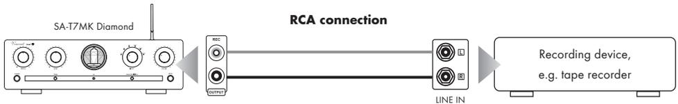
Connect this signal output to the signal input ("LINE IN", "TAPE IN" or "REC IN") on the recording appliance using RCA cables. Please note that some recording equipment can have a slightly detrimental effect on the audio signal quality. Some recording devices have rather low input impedance, which can slightly alter the input signal voltage. For maximal music enjoyment we recommend that you connect to the "REC" terminal only for as long as the recording is actually being made.
