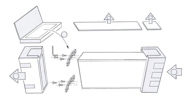
**Caution**: <u>Please carefully put the speaker on its backside, while mounting the base-kit.</u>
