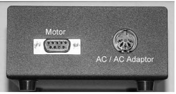
Connect the motorcable with the power pack Ps 800. The backside of the ps 800 offers 1 connector for motor. So plug in the motor cable into the Ps 800 and lock the screws. Make sure that the ON/OFF switch at the front side is in Off
