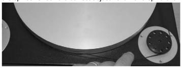
Now place the turntable platter with his axle over the bearing and let it slide into it. Take care that the front end of the axle is not crashing onto the bearing bottom. Then place the rubber belt around the platter and the motor. Now put the feltmat on the platter
