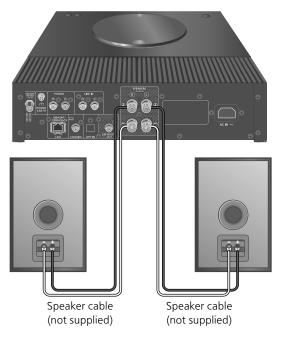
1 Turn the knobs to loosen them, and insert the core wires into the holes.
