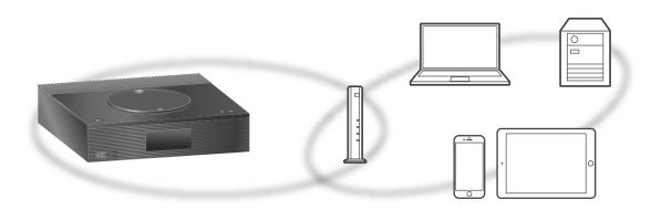
This unit can be connected to a router using a LAN cable or built-in Wi-Fi<sup>®</sup>. For a stable connection to the network, a wired LAN connection is recommended.
