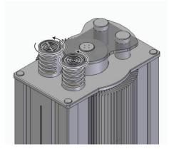
Loosen the tube covers by turning them counterclockwise and then remove them upwards.
