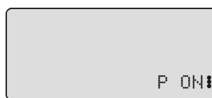
Display in operating condition PROTECT ON
