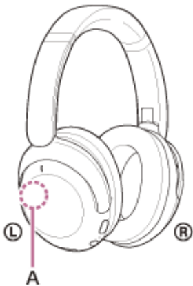
A: Location of the built-in antenna
