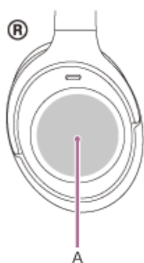
A: Touch sensor control panel
