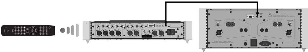
Figure 4: Remote Operation with 12V Trigger
