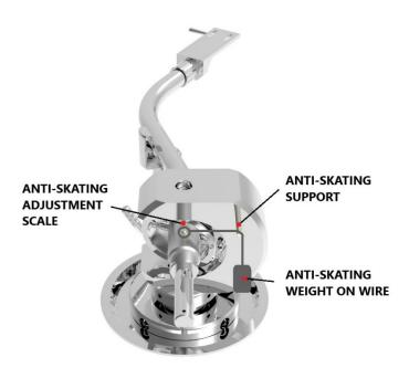
Hang the loop of the thread of the anti-skating weight in the groove of the anti-skating scale (14) corresponding to the downforce applied to your cartridge and hang the thread in the groove of the wire support (15).
