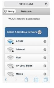
The Stream Box S2 can be connected to a wireless network using any web browser. To do so, connect your mobile device to the integrated Hotspot of your Stream Box S2 (Stream\_Box\_S2\_E690 or similar, depending on each unit).
