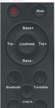
red button turns the unit on or back into standby
