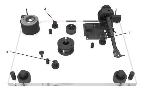
Fit the drive belt (3) around the platter (5) and the motor pulley (2).
