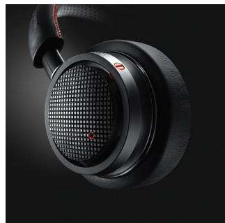
The acoustic closed-back architecture features a Bass Reflex System that comprises ear shells with strategically placed vents. These regulate the air pressure within the internal chamber, providing the diaphragm with a controlled environment for optimal acoustic response. Working in conjunction with the acoustic seal capture, it isolates every natural sound detail and delivers precise and dynamic bass without compromising on sound clarity.
