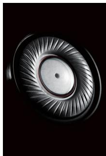
The neodymium drivers respond to all your music's dynamics. The design includes a vent in the centre which emphasises the middle and low frequencies, producing the acoustic energy that brings extended yet controlled bass and a transparent mid-range. The drivers also feature a light voice coil that gives the system nimble response to match the pace of your music and deliver high-definition sound.
