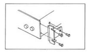
To attach the RMK-800, first remove the three bolts at each side of the cover - closest to the front panel. Use the 6 longer bolts supplied in the rack mount kit to attach both panel extension/chassis supports.
