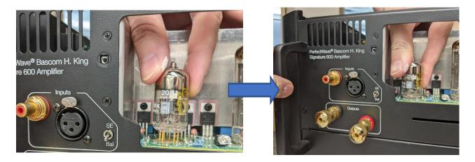
CAUTION/WARNING:REPLACETHETUBECOVERandre-installthetwocoverplatescrews. The tube cover plate must be installed before turning on the amplifier.
