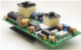
The EB1's 24dB/Oct hand built 31 element precision crossover
