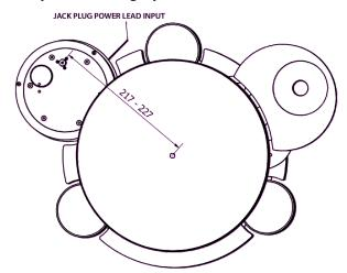
Fit the belt over the platter first and then pull it over the motor pulley taking care not to twist it.
