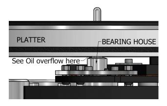
Wipe away excessive overflow at the top of the bearing house but be careful to leave oil clinging to the spindle as you need the top of the bearing to be lubricated by oil overflow and things like tissue paper can suck this area dry by capillary action. You should spin the spindle slowly after it has settled into the bearing to ensure even distribution of oil.
