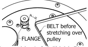
To set correct belt tension finally, lift the belt off the pulley and let it lose it's tension almost completely whilst still holding it gently - With no tension whatsoever in the belt it should be approx 7mm off the nearside of the motor pulley (flange edge) as per diagram below. Move the pod till the pulley is this distance from the belt, then stretch the belt to fit over the pulley.
