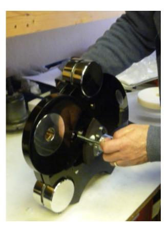
Ensure that the pivot spacer is in position and and then place the sub-chassis over the pivot bolt and ant-rotate stud. These 2 bolts locate the sub-chassis in position. The pivot bolt <u>clamps</u> it and the anti-rotate bolt (loose fit in plinth hole) restrains the whole sub-chassis from rotating out of position. The small hole in the plinth for the anti-rotate bolt is shown in the above illustration.
