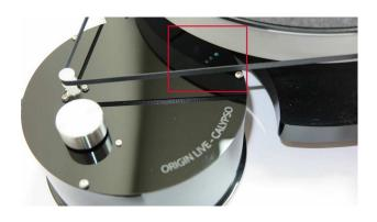
The sensor reads the silver strip on the underside of the platter (see below). This strip must never be removed or the speed will not be correct.
