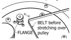
To set correct belt tension <u>finally</u>, lift the belt off the pulley and let it lose it's tension almost completely whilst still holding it gently - With no tension whatsoever in the belt it should be approx 7mm off the nearside of the motor pulley (flange edge) as per diagram below. Move the pod till the pulley is this distance from the belt, then stretch the belt to fit over the pulley.
