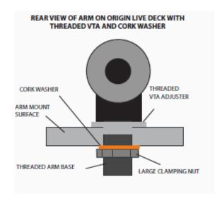
Final setup of tonearm You should refer to your tonearm instructions for detailed set up of arm and cartridge
