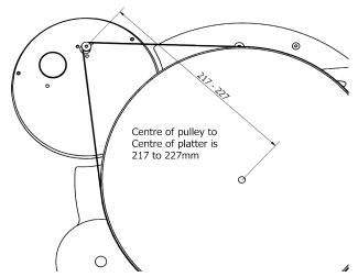
Fit the belt over the platter first and then pull it over the motor pulley taking care not to twist it. To set belt tension, simply move the pod.
