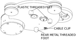
Set the plinth height by rotating the 3 adjustable feet. It helps to lift the deck slightly for access to each foot in turn
