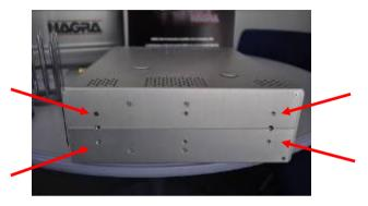
Step 1 Start by removing the transportation screws
