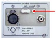
The white jumper allows you to select either XLR balance input (as shown on the picture) or RCA unbalanced
