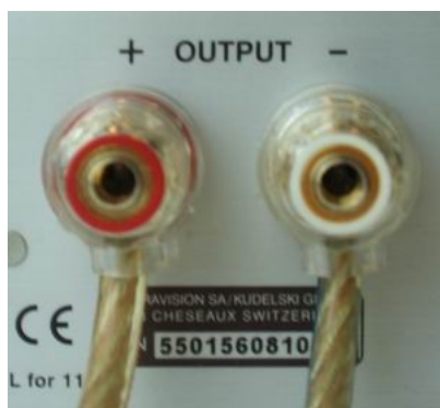
Connecting bare wire cable ends or spade lugs
