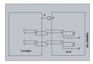
If hum still exists, then verify that the two main power cords (of the PL-P and the turntable) are connected to the mains supply, as close as possible to each other as suggested above in the connection explanation. Floating the earth lead from the turntable may also be tried, as long as the earth connection "X" above is correctly installed.
