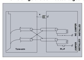
In this case be sure that only ONE of the two jumpers is installed. If you install both jumpers, you immediately have hum again which will be louder or quieter depending on the distance left between the two cables linking the tone-arm with the PL-P. This is explained by the fact that doing this will form a loop which will pickup from magnetic flux adjacent equipment.
