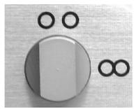
potentiometers are calibrated in logarithmic-scale and represent the amplification of the input amplifier, before the modulometer, for the corresponding channel.
