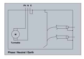
All the various parts of the unit are connected to the chassis and in turn to the earth wire. (This includes the metal parts of the tone-arm as well as the TWO shielding wires of the signal wires coming from the cartridge.)
