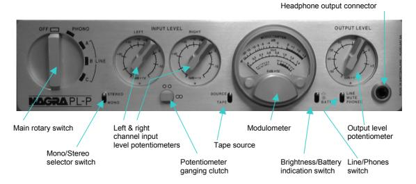
The front panel consists of a variety of controls and a modulometer. Starting at the left of the front panel, they are:
