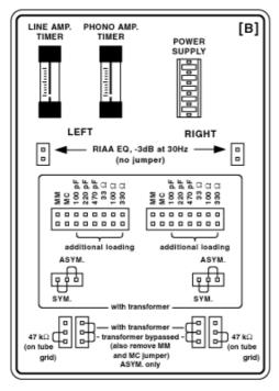
This diagram shows the different jumper positions for the various different options within the PL-P. To install a jumper, place it over BOTH of the pins of the corresponding selection so as to join them together.
