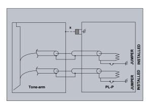
In this third case, both the jumpers are installed and the link between the two chassis "X" is obligatory.
