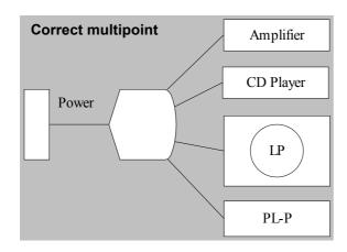
3. A third solution, which is equally viable, is to connect the individual units to the wall connector starting with the highest power consumers and finishing with the lowest power consumer and equally the units using high-level audio signals together and those with lower levels together, as indicated in the diagram below.
