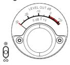
Nagra Modulometer is inherited from the second recorder developed by Nagra back in 1952, the Nagra II. The Modulometer is a typical Nagra precision instrument that displays the necessary information to perform the best possible recording. In the case of the CLASSIC PREAMP, the Modulometer displays the output level. The 0 dB corresponds to a 1 V rms signal on the output.
