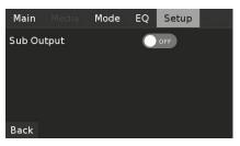
**Sub Output:** At "ON" Setting, all subwoofer settings are in effect. At "OFF" setting, all subwoofer settings are disabled.
