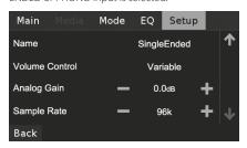
**Analog Gain:** -12dB to 0dB. Gain adjustment allows all sources to play back at the same volume level so you don't need to adjust the volume every time a new source is selected. It is generally preferable to reduce the level of the loudest source rather than making louder the softer sources.
