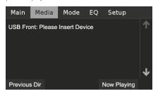
With an external USB mass storage device connected to either USB Front or USB Back input, MP3, WMA or FLAC files or folders will be shown in the touch panel display. Select desired file to playback.
