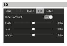
The M12 has the following Tone Control levels – Treble, Bass and Balance. Bass and Treble controls only affect the low bass and high treble leaving the critical midrange frequencies free of coloration. The Balance control adjusts the relative levels of the left and right speakers.
