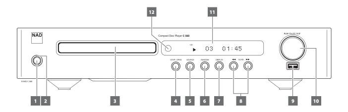
1 STANDBY BUTTON: Press this button to switch ON the C 568. The Standby LED indicator will turn from amber to blue and illuminate the Vacuum Fluorescent Display (VFD). Pressing the Standby button again turns the unit back to standby mode.
