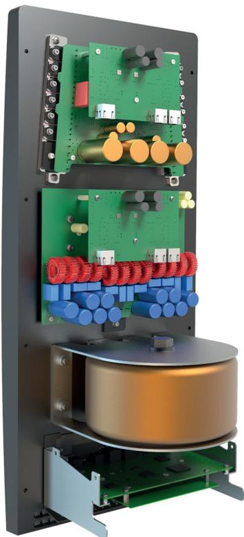
The amplifiers for the tweeter and mid-range driver are Class-AB designs capable of delivering 150W into 4Ω with extremely low noise and distortion under all conditions.
