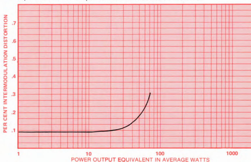
Equivalent Power Output versus Intermodulation Distortion
