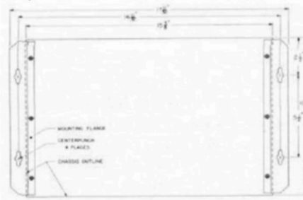
Fig. 4—Bottom of MC240 with mounting flanges attached.
