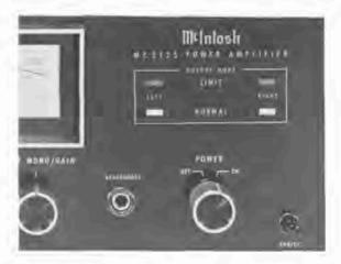
strip on the rear panel. The meter is calibrated for 300 watts at the right hand end of the meter scale. While the MC 2125 cannot reach this power level continuously, it is possible for short interval peaks to exceed, considerably, the 120 watt continuous rating.
